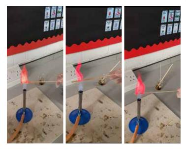
These are some photos from our main three flame tests that we did strontium salt (left), lithium salt (middle) and our soil sample (right). We had to determine which metal cation was present within our soil sample
