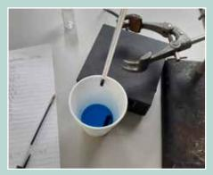
Chemistry practical determining the enthalpy change of reactions.
